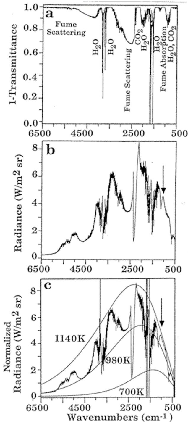
**Figure 2.** Tests of an FT-IR monitor on the recovery boiler of a paper mill revealed that for sub micron fume particles, scattering decreased rapidly with decreasing wavenumber (a), creating partially transparent windows in the spectrum. The experiment also demonstrated that a set of temperature measurements could be derived from the radiance spectrum (b) and from the normalized radiance (c) with a gas temperature of 1140 K, wall temperature of 980 K, and cold gas temperature of 700 K.
