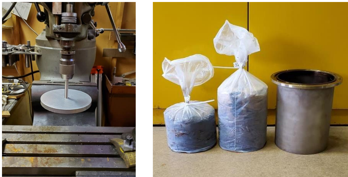
Figure 5. (Left) Photo of the apparatus used for mechanical compaction. (Right) Photo comparing (right to left) a compacted char bag versus an uncompactd char bag and the reactor canister.
