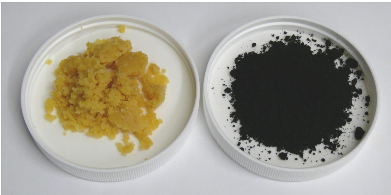
Figure 6. Photograph of a sample of undried fecal simulant (left) and a torrefied (~300 °C) sample (right).
