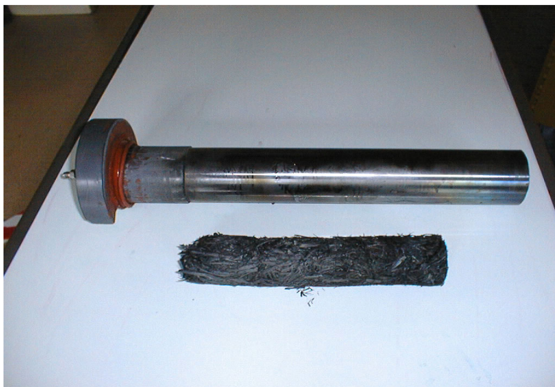
Figure 5. Photograph of new sample holder and charred (unground) wheat straw sample.
